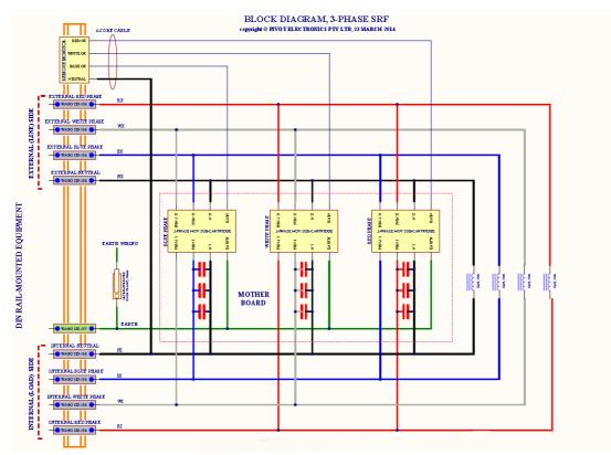
Note: Schematic shown is for TT systems. Neutral Inductor not used on TN systems
